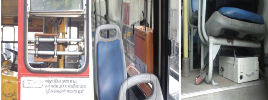
Fig. 5.8 Mumbai trials on BEST Buses (Jan–April 2015): Bus device was mounted on the window and the unit operated with its own battery. The battery unit is seen below the front seat reserved for the disabled
