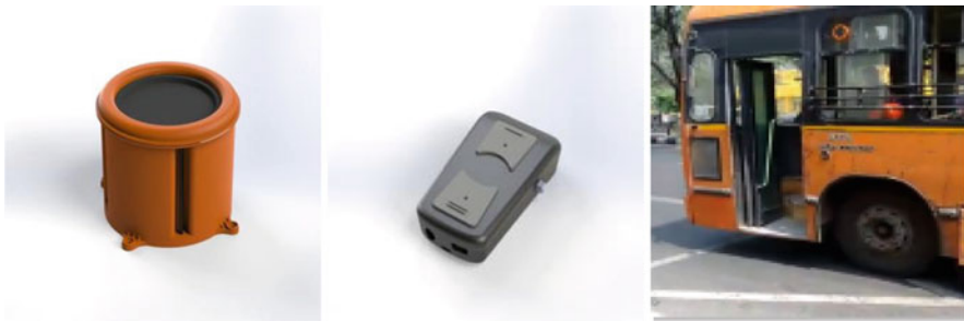
Fig. 5.9 Miniaturized bus device and user device (not to scale) used in the second Delhi trials. The bus device is mounted on the DMITS orange cluster bus in Delhi. Again the validation trials on these new devices were conducted successfully during May to July 2018
