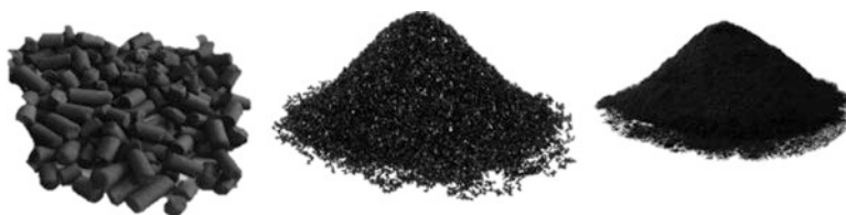
Fig. 1.1 Major classes of activated carbon – (a) extruded or pelletized activated carbon, (b) granular activated carbon, (c) powdered activated carbon (Wikipedia)
