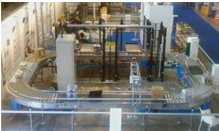
Fig. 18.5 Overall view of the closed-loop roller conveyor in the RFID lab
