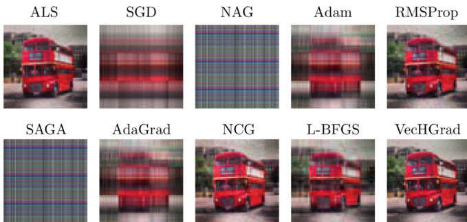
Fig. 4. Visual simulation of the accuracy at convergence of the different optimizers for the PARATUCK2 decomposition. The accuracy is highlighted by how blurry the image is (error at convergence ALS: 1018, SGD: 4082, NAG: 6469, Adam: 2996, RMSProp: 1184, SAGA: 6378, AdaGrad: 2961, NCG: 1569, L-BFGS: 1771, VecHGrad: 599). The popular gradient optimizers AdaGrad, NAG and SAGA failed to converge to a solution close to the original image, contrarily to VecHGrad or RMSProp.
