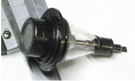
Fig. 11.7 X-ray tube with a glass insulator
