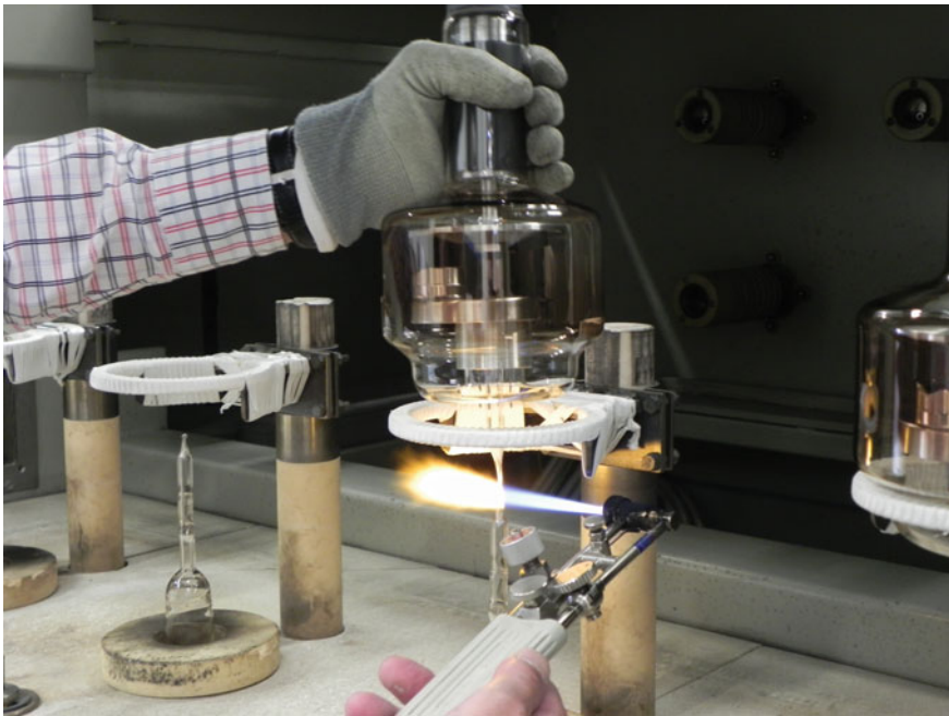
Fig. 5.4 A glass tube for general radiography is pinched-off from the mechanical vacuum pump after the exhaust process is completed. From this point onwards, the vacuum inside the tube is maintained by ion implantation into electrodes and to a smaller extent, by a chemical getter (see Behling [1], Fig. 6.92)
