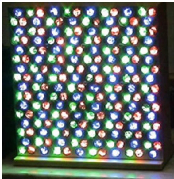
Fig. 10.41 The external module of the full-color video module: 8 by 8 pixels (192) lamp
