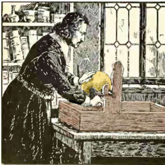
Fig. 1.1 The 1663 electrization machine of Otto von Guericke, using a sulfur sphere and friction. The figure is based on [7], “The electrical experimenter”, Sept. 1915, p.198
