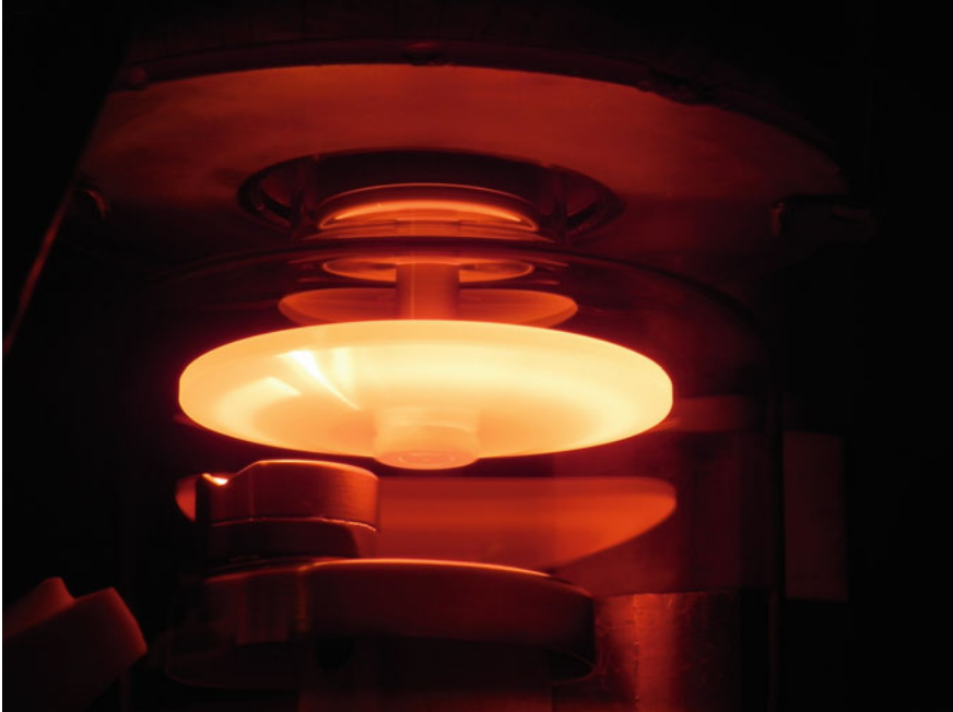
Fig. 5.5 Degassing of a glass tube for general radiography. Electrical power is converted into heat and to a small extent X-ray intensity on the surface of the rectangular focal spot, which leaves a hot comet tail on the focal track. The anode of this sample tube has a diameter of 90 mm and rotates for this picture with 49 Hz. Some visual light from the hot tungsten electron emitter is reflected from the anode as well and visible as a large radial streak parallel to the focal spot
