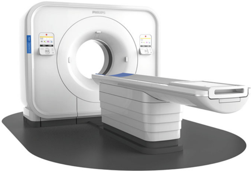
Fig. 5.2 Philips computed tomography system iQon® with spectral detection (“color X-ray”). Polychromatic bremsstrahlung from the X-ray source is attenuated by the patient. In addition to the X-ray intensity, this unique system analyzes the spectrum at the detector downstream of the patient. It enables spectral differentiation between bones, tissue, and contrast agent (iodine). The electron density per volume element of the patient is measured in addition to the attenuation per volume element. In comparison with other concepts, the spectral detection concept delivers the best achievable temporal registration and clinical workflow. Picture courtesy of Philips. Adapted from Behling [1]
