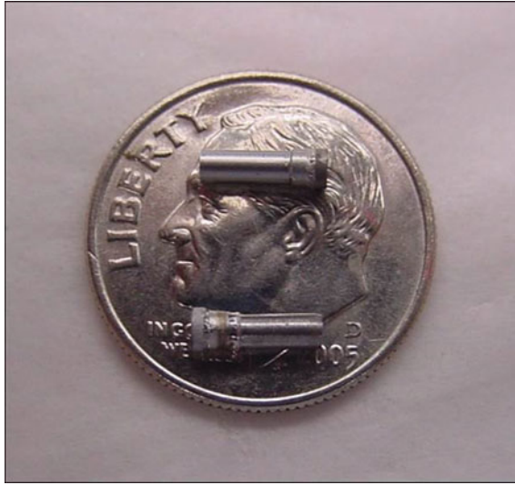
Fig. 2.22 E beam miniature reservoir cathode (bottom) and e beam impregnated cathode (top)
