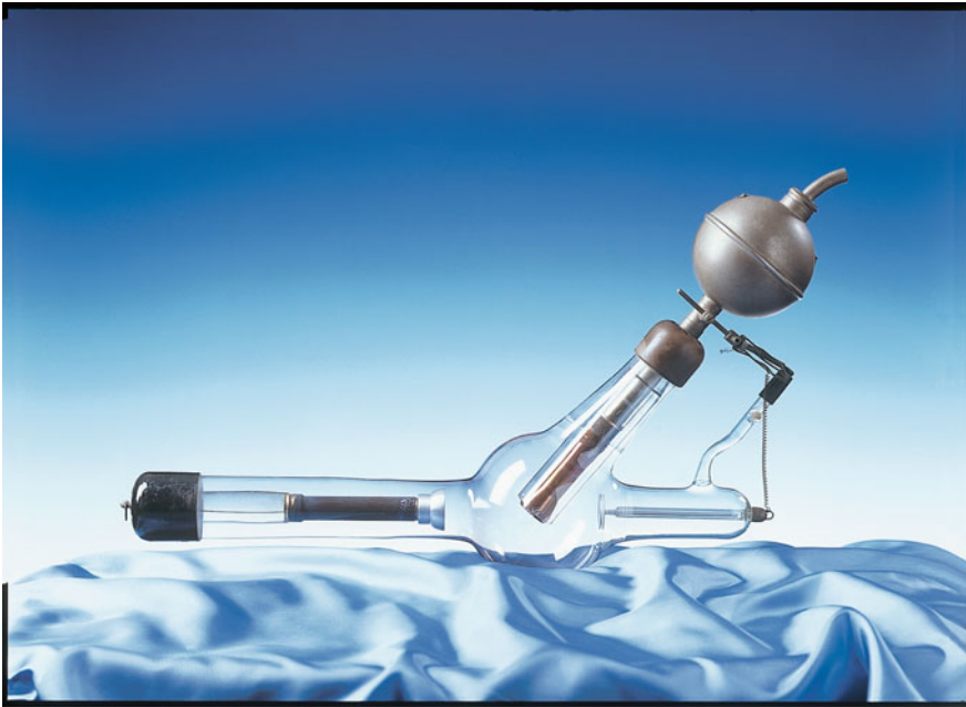
Fig. 5.1 Ion tube with a water-cooled target, manufactured by C.H.F. Müller, Hamburg, ca. 1910 Picture courtesy of Philips
