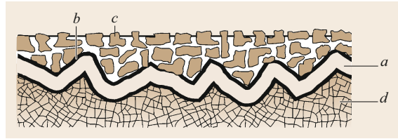
Fig. 9.16 Solid lubrication made of lubricating varnish: a : phosphate layer ( 3\ \mu\text{m} ); b : binder; c : solid lubricant; d : base metal (after [9.15])
