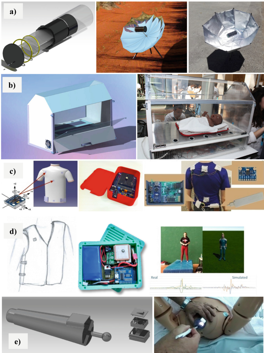
Fig. 3. Examples from medical devices, as result from project-based teaching-learning experiences developed in the “Bioengineering Design” and “MedTech” courses, performed in collaboration between the MSc in Industrial Engineering and the MSc in Organizational Engineering, both at UPM. a) Concept, prototype and experimental validation for a solar powered autoclave for remote settings. b) Low-cost do-it-yourself cradle with autonomous temperature and airflow control. c) System for wrong back posture detection and correction. d) System for detecting falls with wearable sensors driven by artificial intelligence trained with the support of a video game. e) Amnioscope for examining the amniotic cavity tested in delivery simulator.
