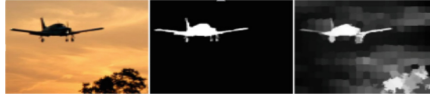
Fig. 4. Initial saliency map. From left to right are input image, GT, Initial saliency map.
