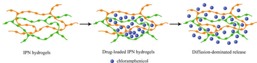
Fig. 13 Schematic diagram of drug loading and release behaviour from the IPN hydrogels [174]. Reprinted with permission from Wang et al. [174] Copyright © 2017 Elsevier
