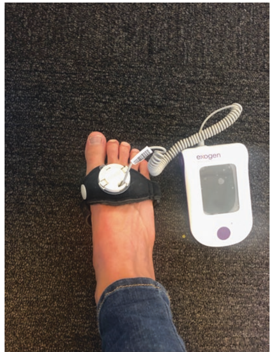
A runner using a low-intensity pulsed ultrasound (LIPUS) device for a second metatarsal stress fracture
