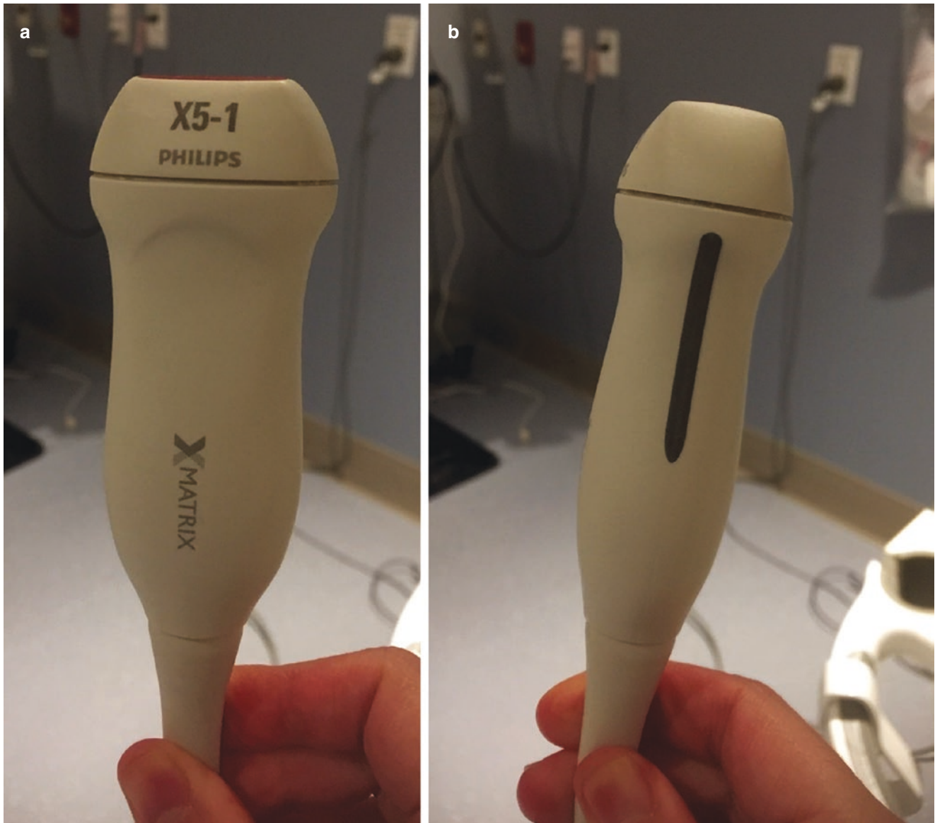
Fig. 2a and 2b Curved linear probe with a small “foot print” viewed anteriorly and laterally
