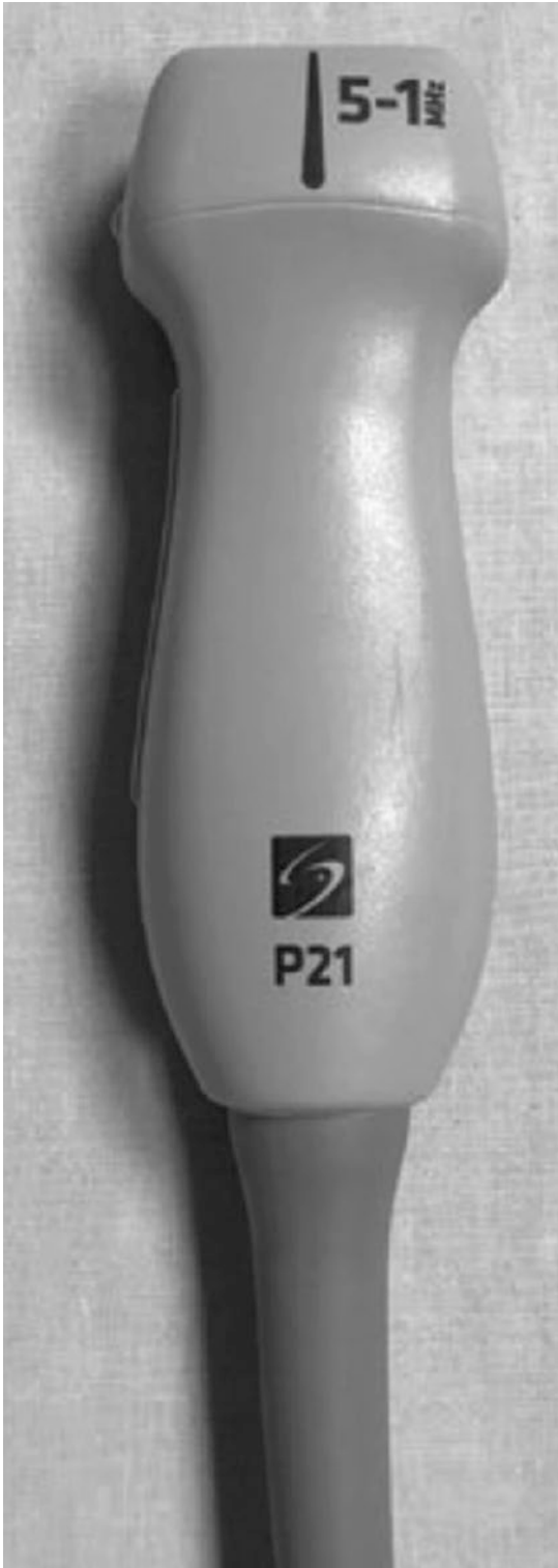
Fig. 4 Phased Array Transducer. (Diagram and adapted caption courtesy of Creditt et al. 2017 Springer)
