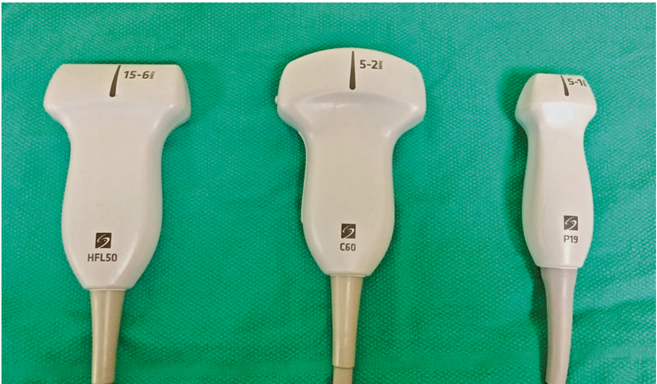
Fig. 1 Examples of common ultrasound probes (left to right): linear probe, curvilinear probe, phased array probe
