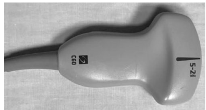
Fig. 3 Curvilinear Transducer. (Diagram and adapted caption courtesy of Credit et al. 2017 Springer)
