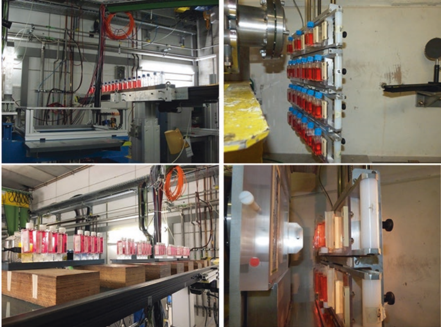
Fig. 1.3 Radiobiological experiments at heavy ion accelerators. Left: 25 cm 2 cell culture flasks and slide flasks filled with medium on the conveyor belt at GSI Helmholtzzentrum für Schwerionenforschung GmbH in Darmstadt, Germany. Right: Irradiation of mammalian cells in 12.5 cm 2 for determination of cell survival and in slide flasks for immunofluorescence staining at the Grand Accélérateur National d' Ions Lourds (GANIL) in Caen, France. In the lower picture, a holder for degraders to modulate beam energy was installed in front of the beam exit window. © Christine E. Hellweg, DLR
