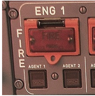
Fig. 4. Engine 1 FIRE push-button on the overhead panel.
