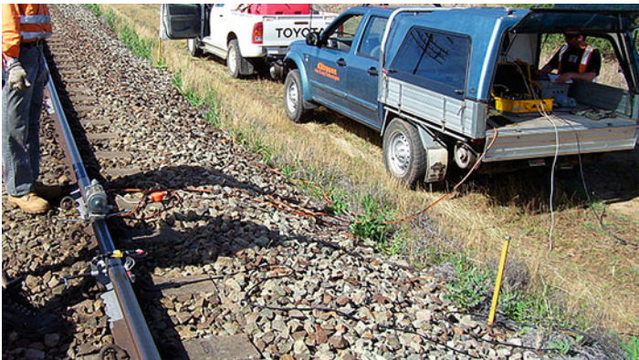
Fig. 3 D'Stresen system mounted on CWR track
