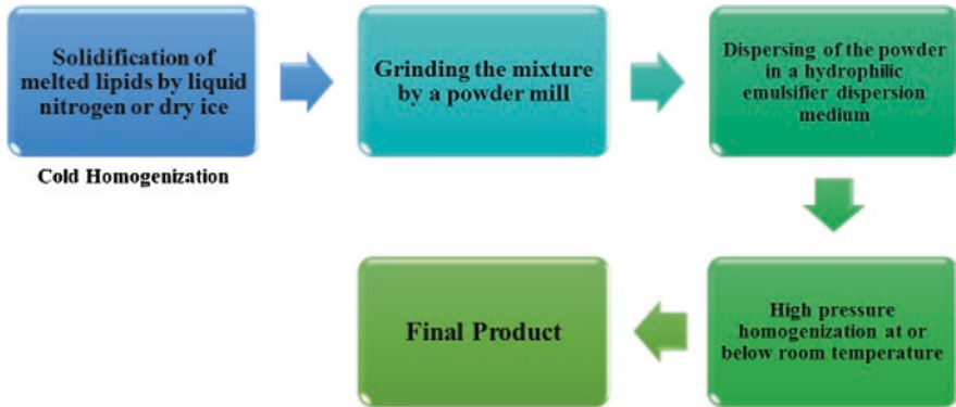
Fig. 8.27 Schematic layout of cold homogenization for NLCs preparation
