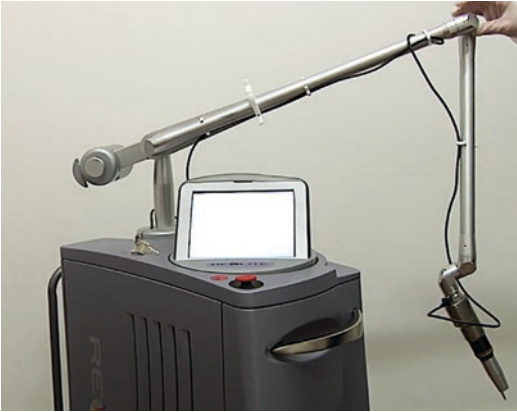
Fig. 1.16 Articulated arm beam delivery system. Courtesy of Cynosure, Inc.
