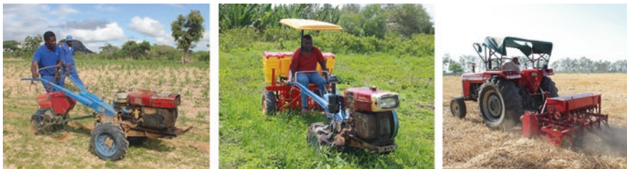
Fig. 28.4 Planting with 2-wheel and 4-wheel tractors with a single row direct seeder (left) a double row direct seeder (middle) and a seeder drawn by a 4-wheel tractor (right). (Photo credits: Baudron, CIMMYT)
