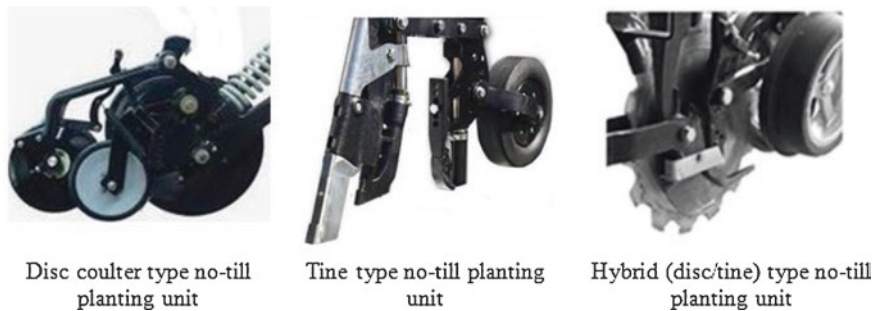
Fig. 6.3 Examples of disc, tine, and hybrid type planting units
