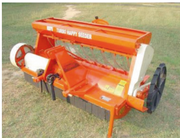
Fig. 21.3 A Turbo Happy Seeder zero-till seeding machine. (Source: Sidhu et al. 2015)
