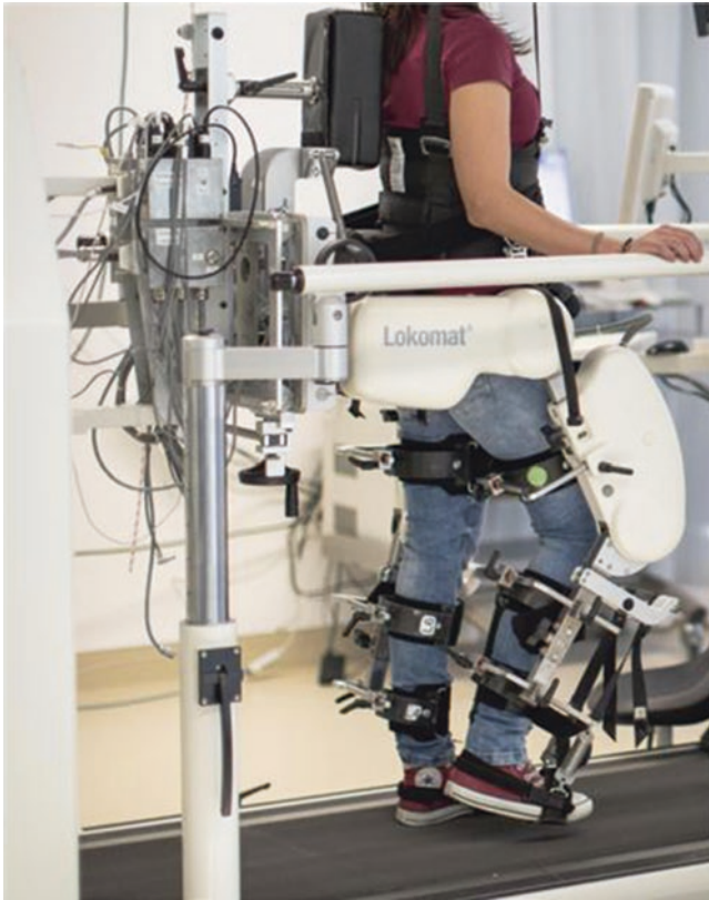
Fig. 4 Person undergoing robotic gait therapy using the Lokomat (Hocoma AG, Switzerland). (Source: © 2018 IEEE. Reprinted, with permission, from Tsangaridis P, Obwegeser D, Maggioni S, Riener R, Marchal-Crespo L. Visual and Haptic Error Modulating Controllers for Robotic Gait Training. 2018 7th IEEE International Conference on Biomedical Robotics and Biomechanics (Biorob), Enschede, 2018, figure 1, p. 1051. Some modifications to the photo were made. doi: https://doi.org/10.1109/BIOROB.2018.8488011 )
