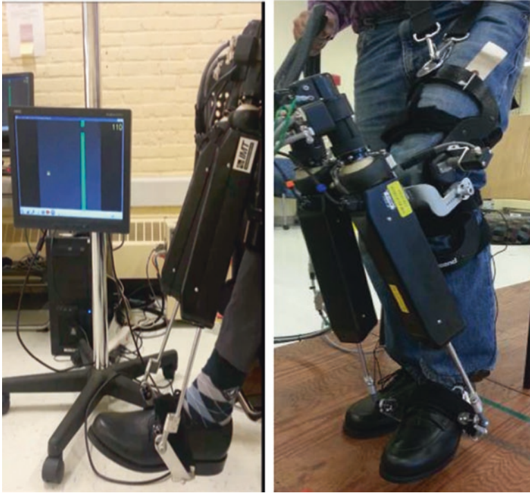
Fig. 7 A two-degree-of-freedom, modular ankle exoskeleton designed to improve ankle function in persons with neurological injuries. Two key therapeutic applications of the robot: seated, computer video-interfaced training (left); overground, robot-assisted gait therapy (right). Key components of the robot include a customized orthopedic shoe and a knee brace that is worn by the subject and secured with quick connectors and a strap attached over the bridge of the subject's foot. The robotic hardware includes two brushless DC motors that drive a pair of linear actuators, which are connected to the shoe using ball joints. A rotary encoder is used to commutate the motor and a linear incremental encoder inside the traction estimates angle. Other peripherals include a potentiometer mounted laterally on the knee to estimate knee angle and a shoulder strap to optionally support the weight of the subject. (Source: United States Patent and Trademark Office. Photo credit: Anindo Roy)
