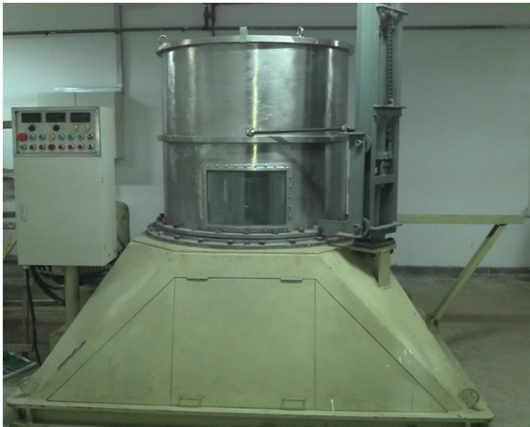
Fig. 3. The Cylindrical Erosion Test Apparatus (CETA).
