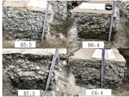
Fig. 4. The typical sections of the shear specimens
