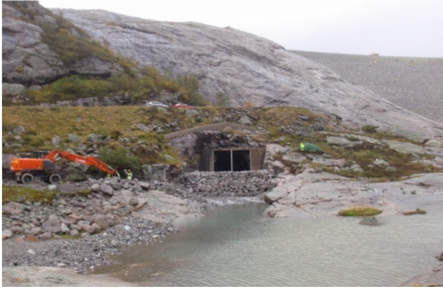
Fig. 3. Field site for the large-scale riprap tests. The 3 m high and 12 m wide test dams were situated in the outlet channel (in the center) of the large dam Svartevatn (in the background on the right). (Photo of test F13P1: NTNU)
