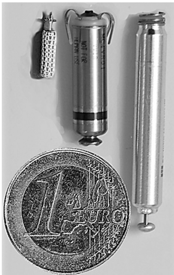
Fig. 10.3 Composite representation of the three commercially available leadless PM ( demo versions ). For the Wise™-CRT (Wireless Stimulation Endocardially for CRT; EBR Systems Inc., CA, USA) pacing system only the intracardiac component is represented
