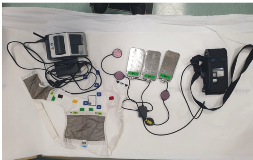
Fig. 7.3 All components of a LifeVest® (Zoll)—wearable cardioverter defibrillator—before applied to a patient
