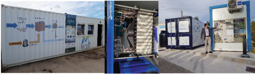
Fig. 5. The MIDES pilot Microbial Desalination Cell (MDC) in Dénia Demo-site.
