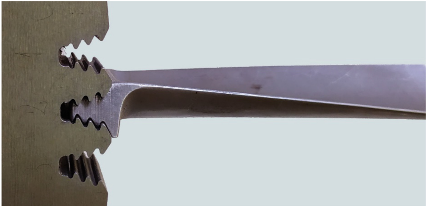
Fig. 10. Turbine blade positioned in the auxiliary tool
