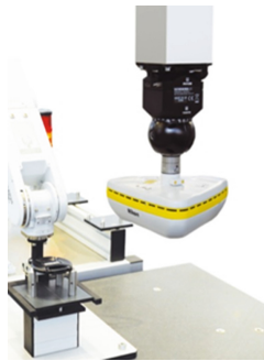
Fig. 3. Robotized CMM equipped with laser triangulation scanner cooperates with industrial robot [15]
