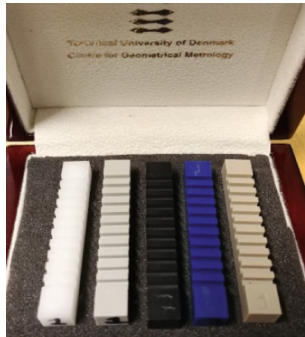
Fig. 10. Polymer step gauge used in [2].
