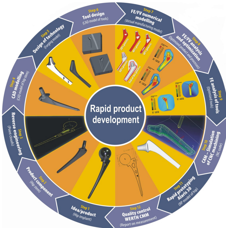
Fig. 3. Integrated MBM approach in design of customized implant and its fabrication processes
