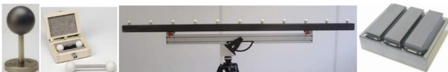
Fig. 2. Standard reference objects for testing optical based scanners [16].
