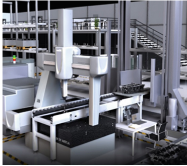
Fig. 4. Automation of CMM measurements using automatic feeder [15]
