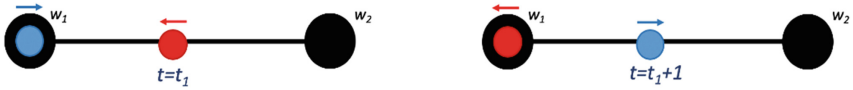
Fig. 3. Case3(a). A collision occurs when two agents try to swap their places along a slow edge \langle w_1, w_2 \rangle and one of them is a bit ahead in transit.
