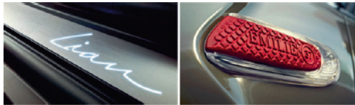
Fig. 1. An example for customized parts of an automobile with AM: led door sills and side scuttles of BMW MINI 2018 [15]
