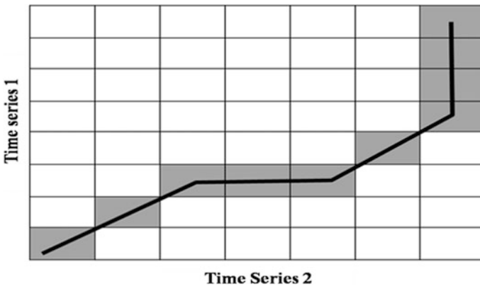
Fig. 5.5 Minimum-distance warp path
