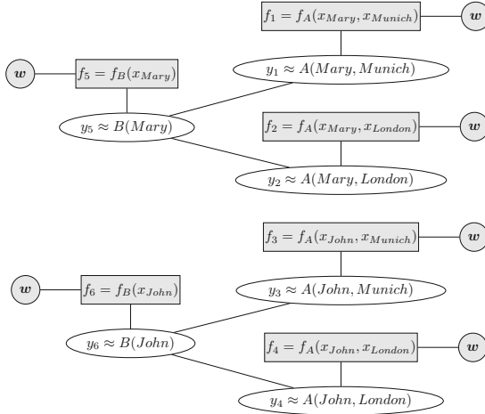
Fig. 2. The undirected graphical model built by a DLM for the rule \forall v_1 \forall v_2 \neg A(v_1, v_2) \wedge B(v_1) where v_1 can assume values over the constants \{Mary, John\} and v_2 over \{Munich, London\} . Each stochastic node y_i approximates one grounded predicate, while the f_i nodes are the actual output of a network getting the pattern representations of a grounding. Connections of all latent nodes y_i to the parameters \lambda have been omitted to keep the picture readable.
