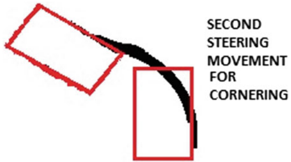
Fig. 12.7 Vehicle movement after the second steering position during parallel parking
