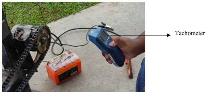
Fig. 15.5 Alternator's speed reading measurement
