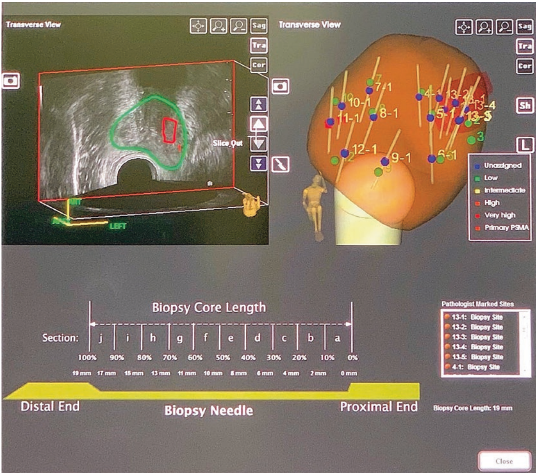
Fig. 10.3 A longitudinal view of the output from Artemis fusion platform. The target lesions are volume-rendered, while the lines show the biopsy needle positions. The center of the biopsy needle where the cores were obtained is
