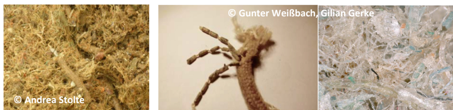
Fig. 3. Left: Shredded gillnets with residual sink lines, the lead fragments showing at the centre of the image (© Andrea Stolte). Middle: Sink line with lead pieces embedded in PET sheathing (© Gunter Weißbach, Gilian Gerke). Right: Microscopic image of fibre mix showing twists and bents that cause contaminants to be trapped (© Gunter Weißbach, Gilian Gerke).
