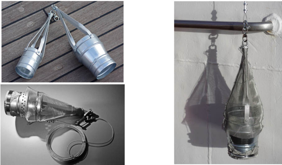
Fig. 1. The metal filter support with the front chassis at different stages of device construction.
