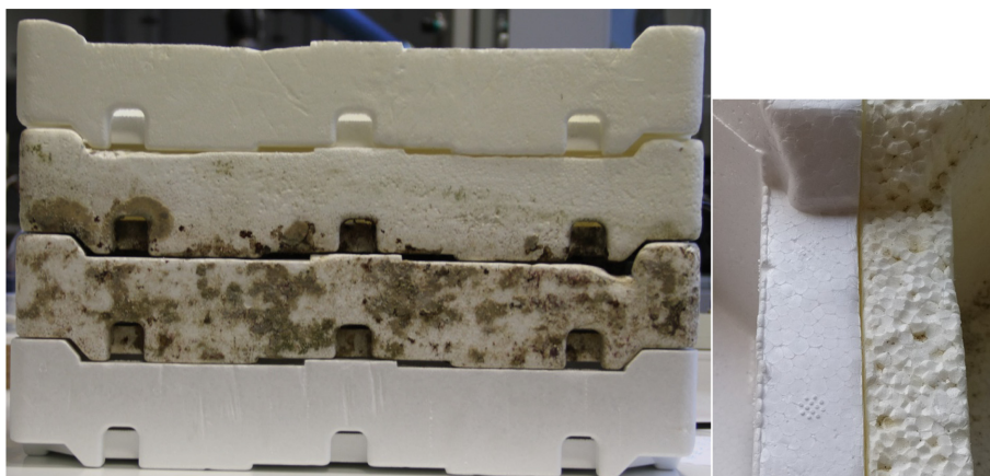
Fig. 7. Right: lateral view of the EPS samples (Blank, 9MF, 9MS and S from bottom to top). Left: upper border of the EPS box before and after 9 months of aging in sandy shoreline (corrugation effects).
