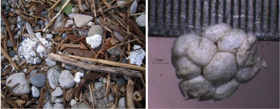
Fig. 4. EPS particles at different level of fragmentation
