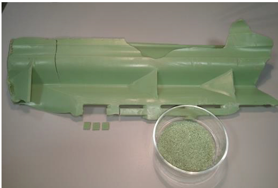
Fig. 8. HDPE-fragment #4 (weight 788 g; length 53 cm) retrieved in Zone 2B. (November 3 rd , 2018). Three specimens for Vicat test and grinded parts for MFI analysis are showed.
