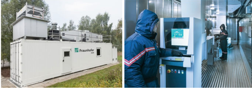
Fig. 13 Ice Wind Tunnel test facility of Fraunhofer IFAM. Published with kind permission of © Fraunhofer IFAM 2016. All rights reserved
