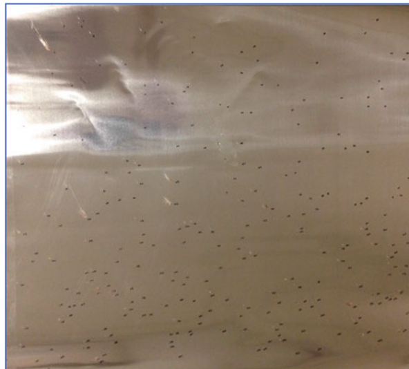
Fig. 3 Insect residue accretion location on uncoated aluminum panel
