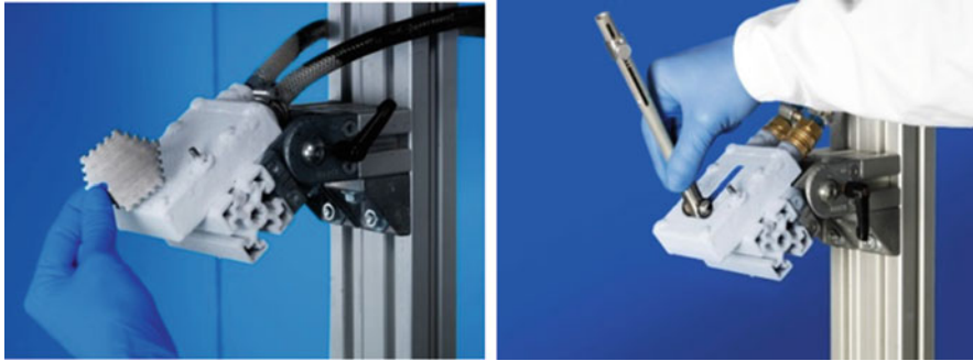
Fig. 4 Rime ice test in Fraunhofer IFAM Ice Chamber: thickness measurement with film thickness gauge ( left ) and adhesion measurement with modified mar resistance tester ( right ). Published with kind permission of © Fraunhofer IFAM 2016. All rights reserved
