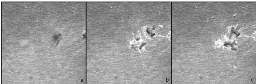
Fig. 8 Image sequence of D. melanogaster . (Test facility: SPIrIT, specimen: 15, substrate temperature: 20°C, impact angle: 90°, impact velocity: 100 m/s). (a) Insects approaching the test plate. (b) Insects impacting the surface. (c) Insect residue spreading on the surface
