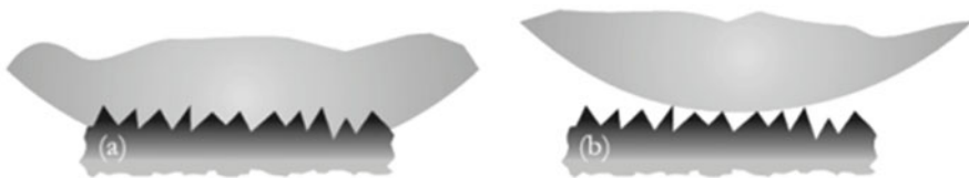
Fig. 8 Schematic representation of the two different cases of wetting on rough surfaces: (a) the Wenzel-regime; (b) the Cassie–Baxter regime. From Stenzel et al. [10]. Published with kind permission of © Fraunhofer IFAM 2016. All rights reserved
