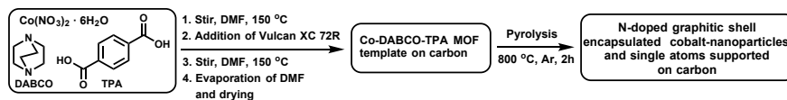
Fig. 6.4 Preparation of cobalt nanoparticles and single atom-based catalysts by the pyrolysis of Co-MOF on carbon
