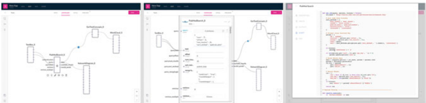
Fig. 13 Connection-level dataflow (left), Configuration-level dataflow (middle), Code-level dataflow (right)
