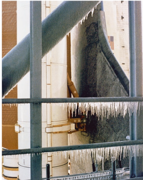
Fig. 11.1: (top) The STS-51L crew in the White Room at KSC Pad 39B during training. [l-r] PS Christa McAuliffe, PS Greg Jarvis, MS and TFNG Judy Resnik, CDR and TFNG Dick Scobee, MS and TFNG Ron McNair, PLT Mike Smith, and MS and TFNG Ellison Onizuka. (bottom) The build-up of ice on Pad 39B is evident in this image. Challenger , the ET and the left-hand SRB are in the background.
