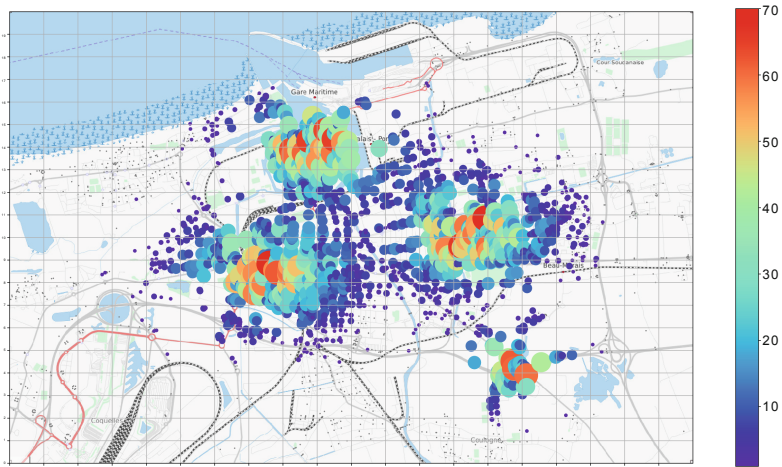
Fig. 2. Four home clusters inside Calais road network. Colors indicate the number of agents departing from a node. (Color figure online)
