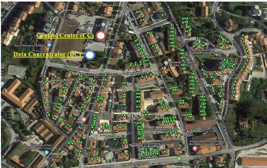
Fig. 3. WaterAMI solution installed in CELBI's M&CS: each green point signs out one WWMT, i.e., a network node (Color figure online)
