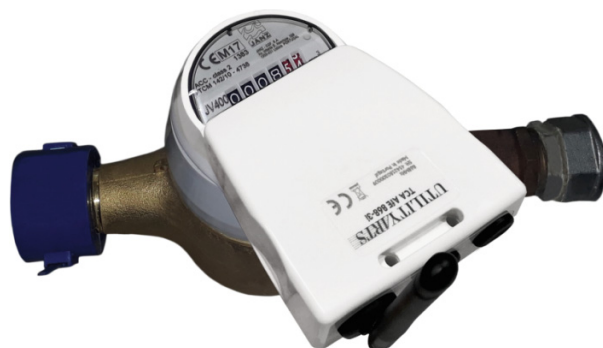
Fig. 2. The WaterAMI is composed by a Wireless Water Metering Transceiver (WWMT), powered by standard non-rechargeable/depletion batteries, prompt to be installed in conventional water meters (e.g. JANZ JV400). After, reading the data with an incremental encoder, the WWMT sends the data collected through AfE-EA communication protocol to DC.
