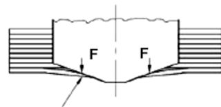
Thrust and rotate action of cutting edge
