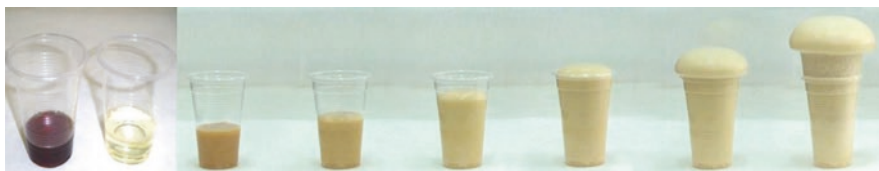
Fig. 5.1 The isocyanate, the polyol and the foam formation after mixing of them
