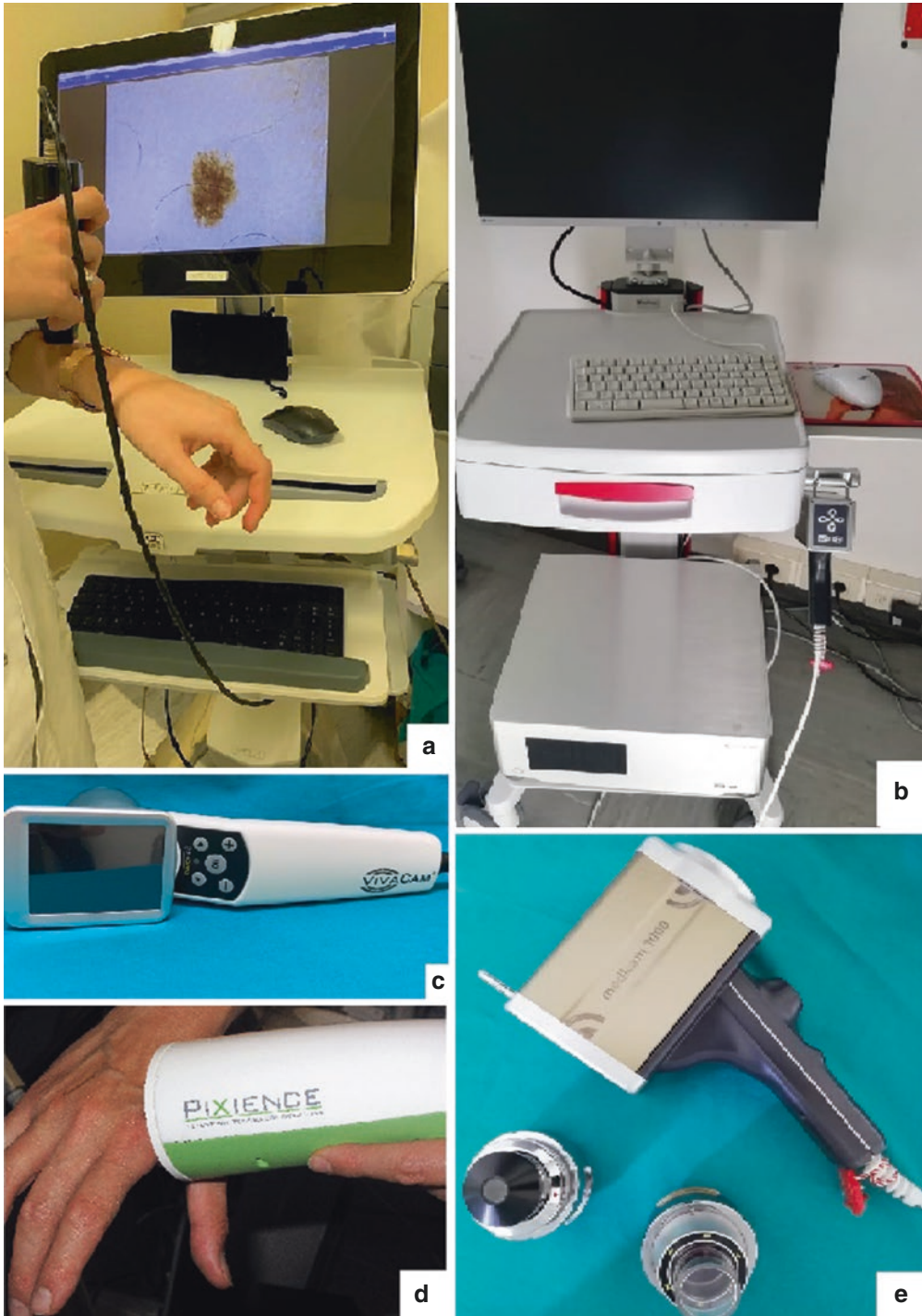
Fig. 1.4 Different models of video dermatoscopes, using different probe camera and software: Horus HS600 (Adamo SrL, Italy) (a), FotoFinder (Fotofinder Systems GmbH Bad Birnbach, Germany) (b), VISIOMED D200EVO (Canfield, Canfield Imaging Systems, Fairfield,
