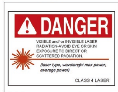
Fig. 29.2 Laser warning signs to be positioned outside the laser-controlled area (IEC 60825-1 for EU zone and ANSI Z136.1 in the USA)
