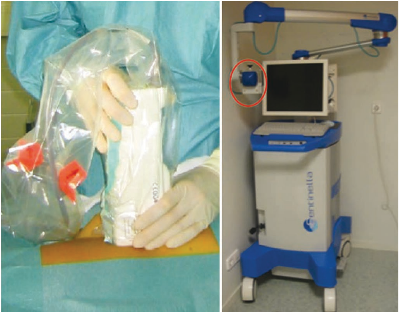
Fig. 7.10 Example of portable gamma cameras. Left panel: light-weight portable gamma camera (less than 1 kg), without support system. Right panel: recent-generation portable gamma camera with
