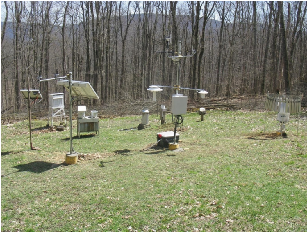
Fig. 9.7 Smart sensor array monitoring of soil and atmospheric properties in real-time. (Photo credit: Ian Halm, USDA Forest Service)
