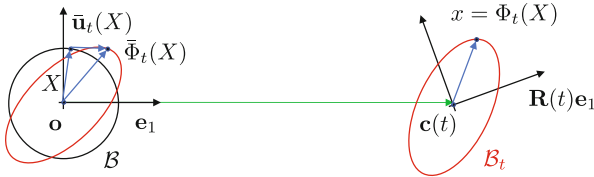
Fig. 1.1 Reference and deformed configurations of a swimmer: parametrization of the swimmer motion in terms of position \mathbf{c}(t) , orientation \mathbf{R}(t) , and shape \bar{\Phi}_t . Figure reproduced from [35]
