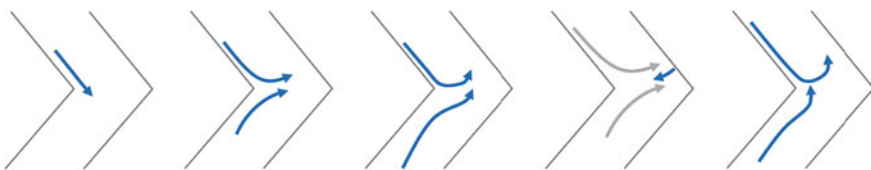
Fig. 9 Dominating particle trajectories identified by shadowgraphy along each bend of the zigzag channel
