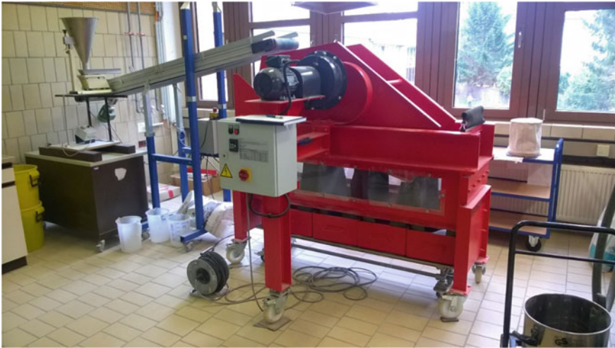
Fig. 34 Circular vibratory screening machine (Rekord V 3/10/I L of Siebtechnik GmbH)
