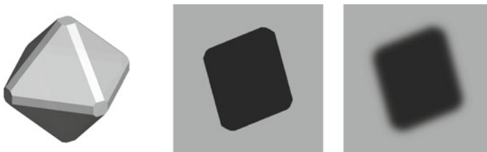
Fig. 3 Rendered 3D model of a potash alum crystal model with 26 faces (left), a 2D projection of this crystal (middle) and the same 2D projection to which blur was added (right). (Reprinted with permission from [9], Copyright (2015) Elsevier)
