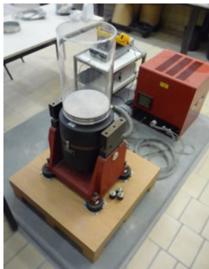
Fig. 27 Experimental set, electrodynamic vibration exciter
