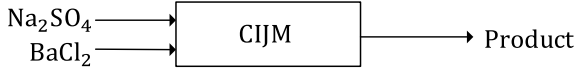
Fig. 8 Simulation flowsheet for steady-state model validation (Setup A). Reprinted with permission from [5]
