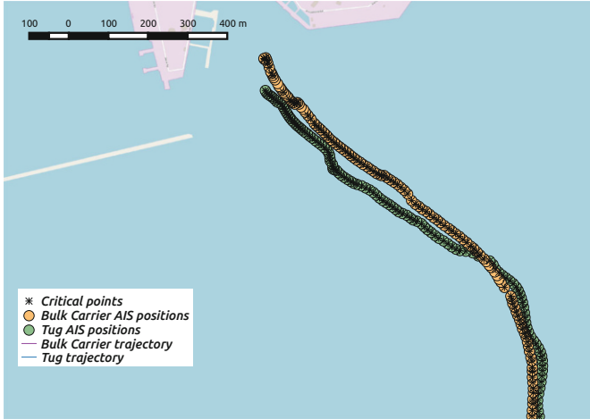
Fig. 9.8 Example of bulk carrier tugging. In this example, all position signals are labelled as ‘critical’
