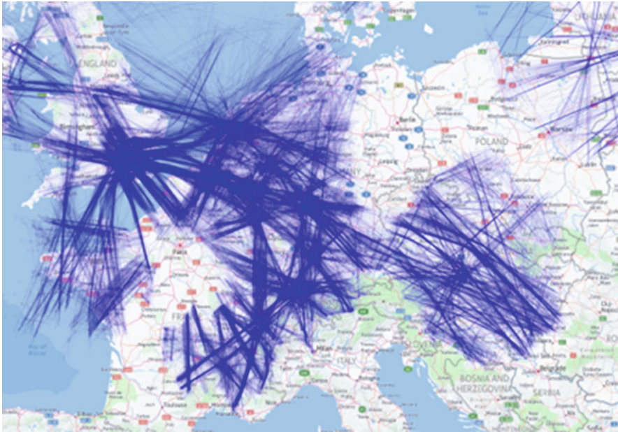
Fig. 3.4 An example of problems with spatial coverage in a dataset with aircraft trajectories
