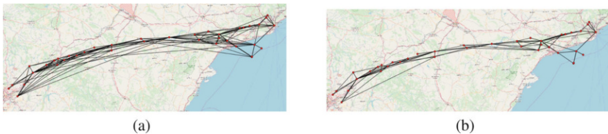
Fig. 10.15 Discovering paths (edges) of the network, (a) all edges found with weight over 0 (182), (b) keep only edges with weight over 2 (130)
