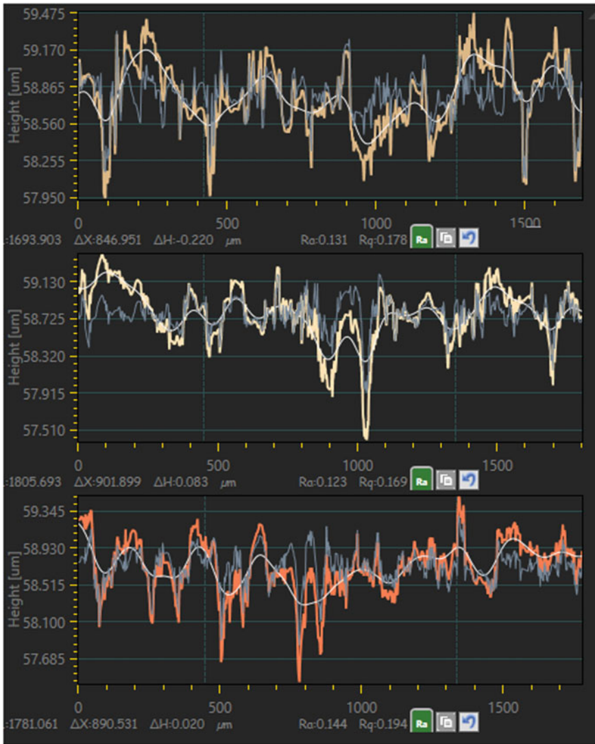
Fig. 22.8 Plot of the surface roughness of the sample with optimized parameters
