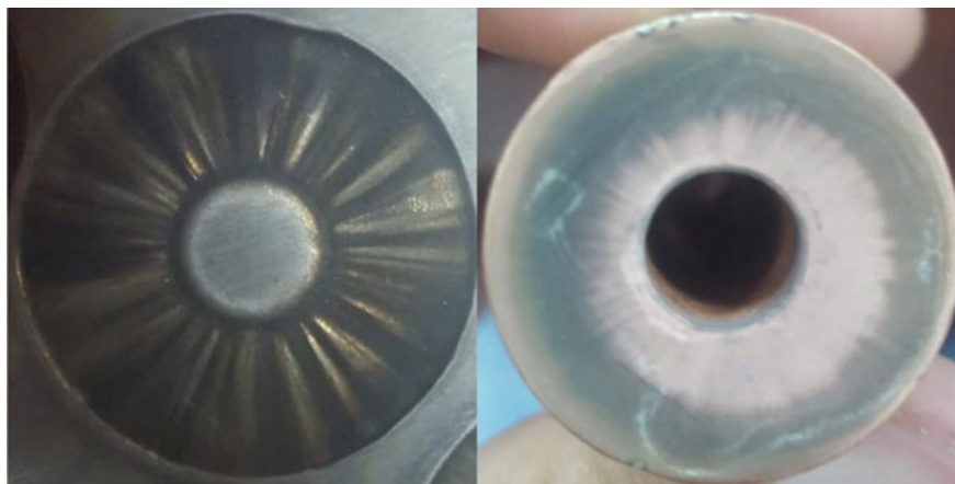
Fig. 22.5 Sample surface of high roughness surface (left) and the surface of electrode after manufacturing (right)
