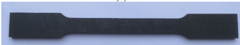
Fig. 9.1 Tensile test specimen: a dimensions, b wire cutting by CNC and c final shape
