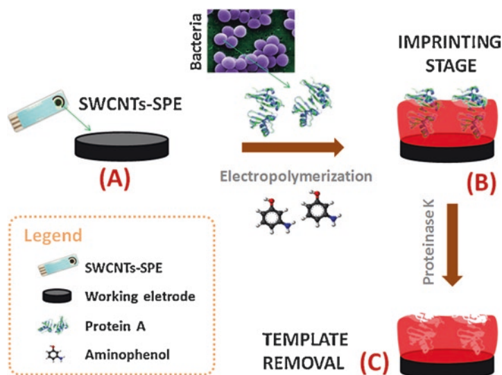
Fig. 13 Schematic representation of the synthetic process. (a) Working area of SWCNTs-SPE; (b) Imprinting stage after electropolymerization of AP along with PA and (c) Binding site formation after template removal by proteinase K (Reprinted with permission of Khan et al. 2016)
