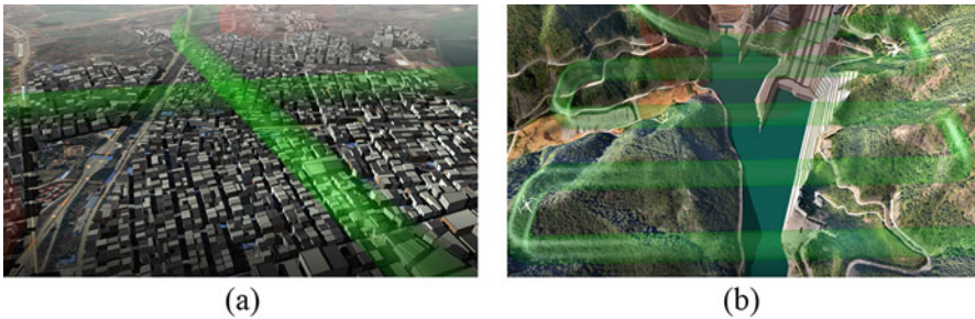
Fig. 4 Visualized scene of UAS flight area with an aerial corridor. (a) Aerial corridor in an urban area. (b) Aerial corridor in rural area
