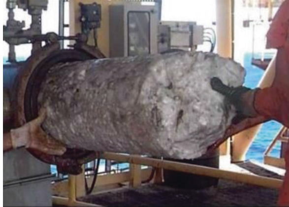
Fig. 11.3 Hydrate plug formed in subsea pipeline
