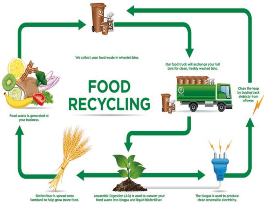
Fig. 16.15 Recycling of food waste into electricity
